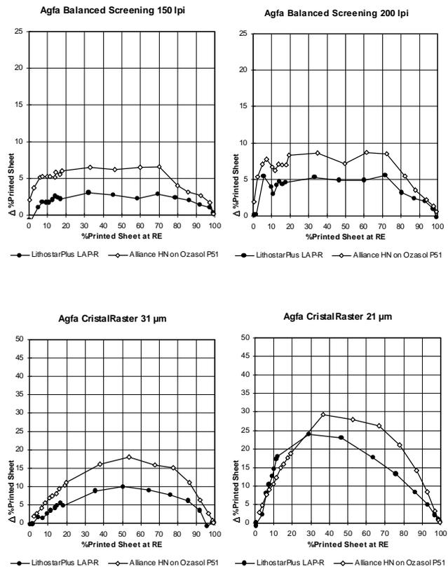
Figure 9 : Difference in tone reproduction on the printed sheet between underexposed (-0.15logH) and overexposed media (+0.15logH) (relative to the tone reproduction at the right exposure)
