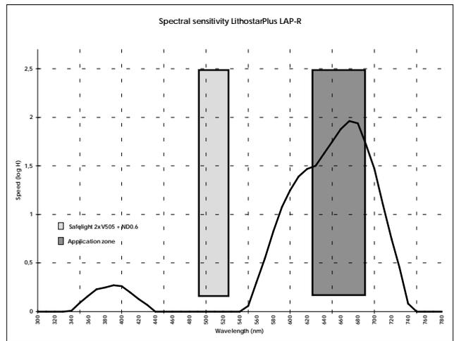
Figure 7 : Spectral sensitivity curve of LAP-R
