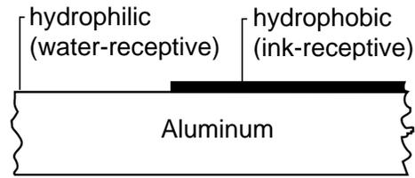
Figure 6: Finishing or gumming step
