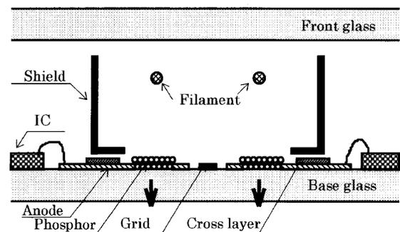
Figure 2 Electrode Structure of VFPH
