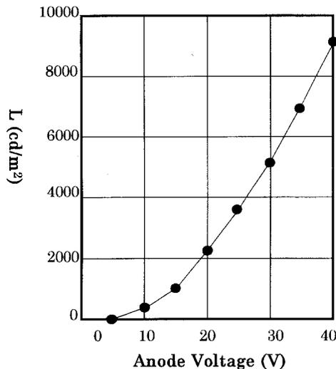
Figure 4 Relationship Between Luminance and Anode Voltage
