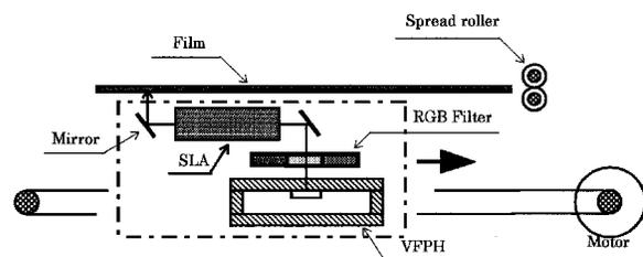
Figure 1 Structure of Printer
