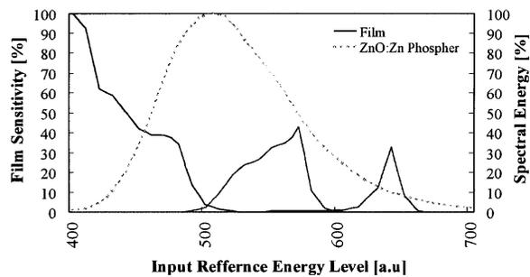
Figure 6 Film Sensitivity and ZnO:Zn Spectral Energy
