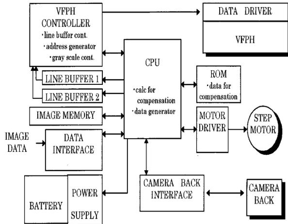
Figure 7 Block Diagram of Printer System
