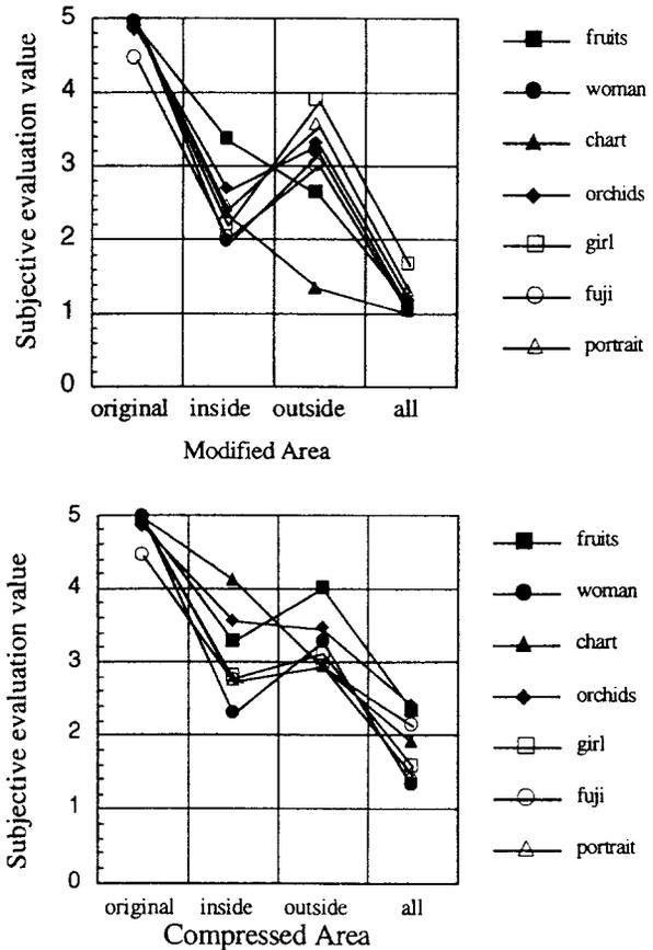
Figure 4. Subjective evaluation of blurred (a) and compressed (b) inside of gazing area, outside gazing area and entire of the image for seven kinds of images.
