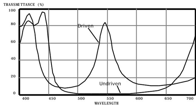
Figure 9 STF for a transmissive IMod design showing Driven and Undriven states.
