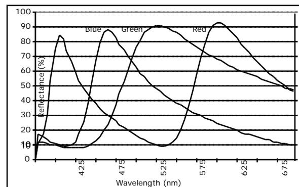
Figure 5 Spectral Reflectance Functions (SRFs) of measured IMod tests at increasing Color/Gap dimensions: green (160 nm), blue (300 nm) and red (400 nm).
