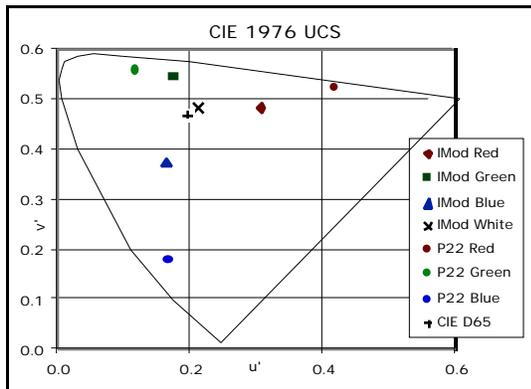
Figure 7 Measured color gamuts of IMod color display triads compared to P22 phosphors using CIE 1976 UCS.
