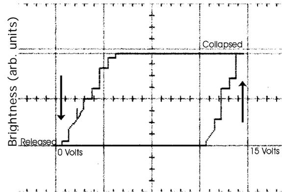
Figure 4 Plot of drive voltage vs. output magnitude revealing hysteresis of the IMod.
