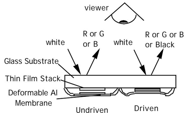
Figure 1 Illustration of the basic structure of a reflective Interferometric Modulator (IMod).
