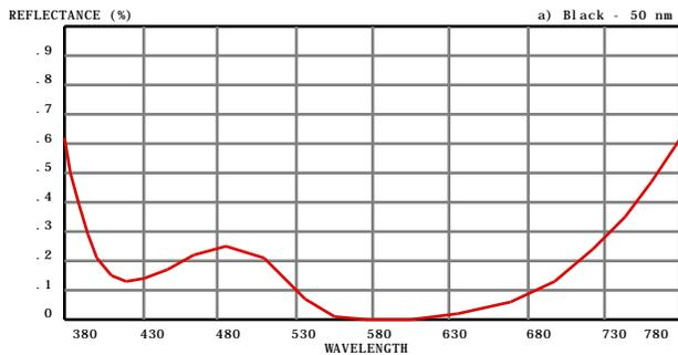
Figure 3 Reduced scale plot of SRF of calculated black Color/Gap dimension.
