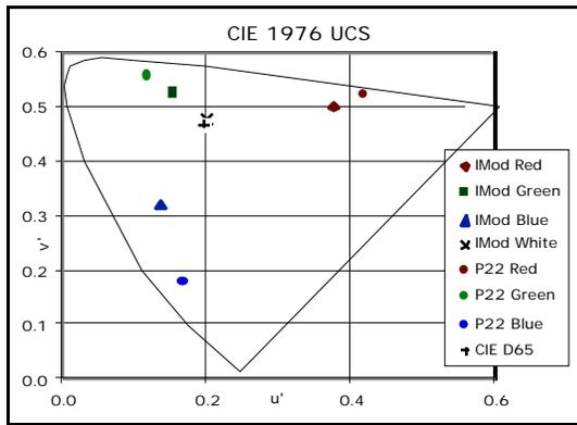
Figure 6 Calculated color gamuts of IMod color display triads compared to P22 phosphors using CIE 1976 UCS.
