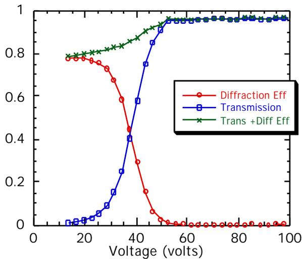
Figure 1: Electric field switching of a transmission grating studied by applying a square wave across the PDLC grating.
