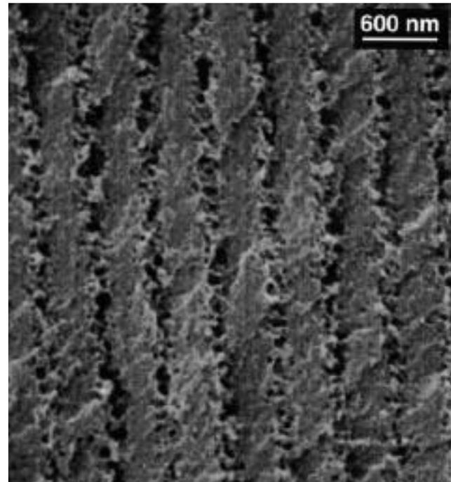
Figure 2: Morphology of a PDLC transmission grating (edge view).
