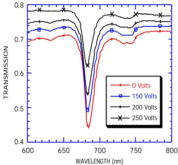
Figure 3: Transmittance of a PDLC reflection hologram.
