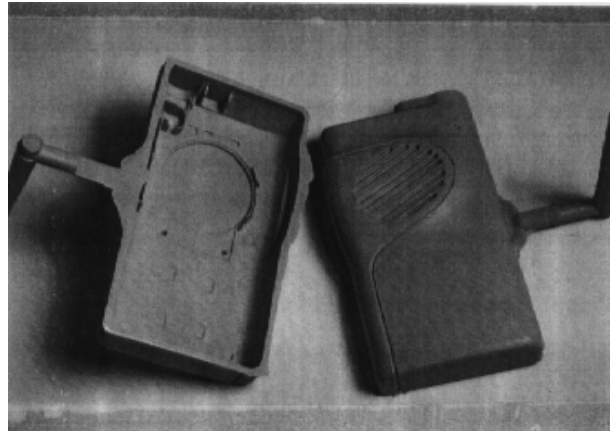
Figure 1. Cavity and Core insert set directly from the epoxy bath material
