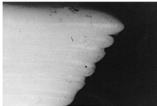
Figure 3. Edge scalloping effects resulting from light scattering in an alumina resin cured with an argon ion laser.
