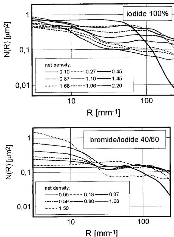
Figure 6. Wiener spectra at varying densities for collodion containing only iodide (a) and bromide/iodide (b).
