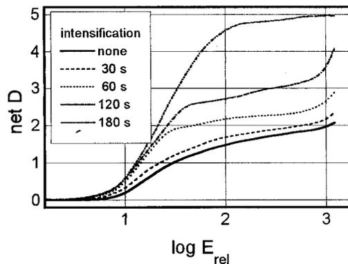
Figure 7. Characteristic curves of the wet collodion process with varying intensification times.
