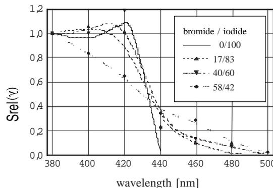
Figure 4. Distributions of relative spectral sensitivity for varying bromide/iodide molar ratios.
