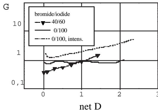
Figure 5. Selwyn granularity  $G$  as a function of density.
