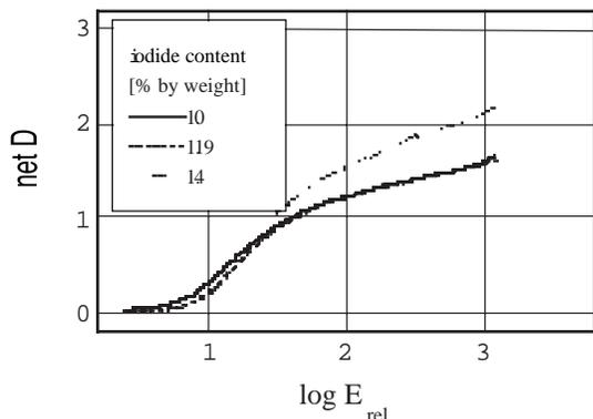
Figure 2. Characteristic curves of the wet collodion process for varying iodide concentrations.
