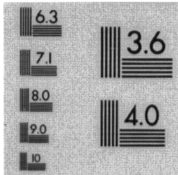
Figure 2. 600 dpi scan of microcopy resolution test target resolved 9.0 line pairs per millimeter.
