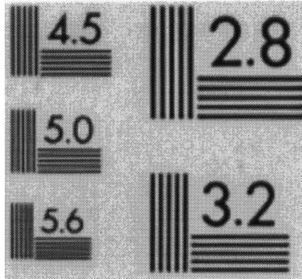
Figure 1. 300 dpi scan of microcopy resolution test target resolved 4.5 line pairs per millimeter.
