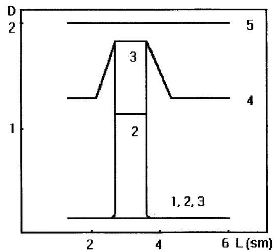
Figure 1. Effect of cathode potential on selectivity of electroreduction of grains of undiluted positive emulsion. Relative potential values: 1-0,25 (absence of reduction); 2-0,5 (onset of reduction of exposed (grains)); 3-1,0 (complete and selective reduction of grains at slower rate); 5-6.0 and higher (non-selective reduction of latent image specks).
