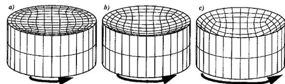
Figure 2. Sample predictions of 3D free surfaces of a fluid under solid-body rotation with angular velocities that cause vertical displacements of a)  $\Delta z = 0.05$  b)  $\Delta z = 0.25$  c)  $\Delta z = 0.5$ .
