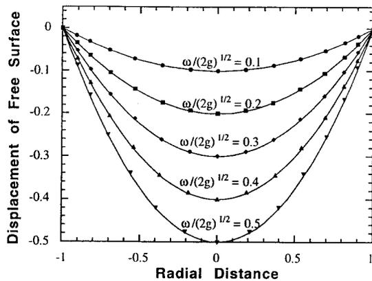
Figure 3. Comparison between free surface shape predicted by 3D Computational Fluid Mechanics (symbols) and the analytical result (lines) for a fluid in solid-body rotation.
