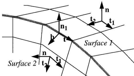
Figure 1: Illustration of the issues surrounding rotation of mesh equations on surfaces and edges.
