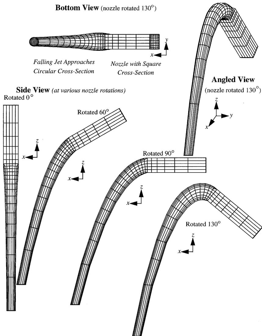
Figure 4. Sample predictions of fluid extruding from a nozzle of square cross-section and bending under gravity.  $\rho = 1 \text{ gf/cm}^3$ ,  $\mu = 1 \text{ poise}$ ,  $\sigma = 30 \text{ dynes/cm}$ ,  $g = 980 \text{ cm}^2/\text{s}$ ,  $w_{\text{nozzle}} = 0.5 \text{ cm}$ ,  $Re = 12.5$ ,  $Fr = 10.2$ ,  $Ca = 1.7$ ,  $v_{\text{max, nozzle}} = 50 \text{ cm/s}$ .
