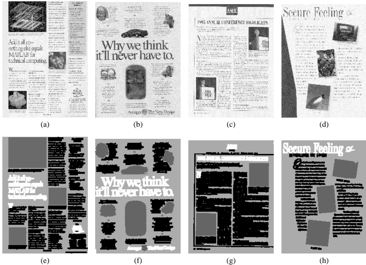
Figure 9: Training images and the corresponding “ground truth” segmentations: (a)-(d) are training images, and (e)-(h) are “ground truth” segmentations. The dark areas are text, the dark grey areas are images, the light grey corresponds to background, and the white areas are the headings.
