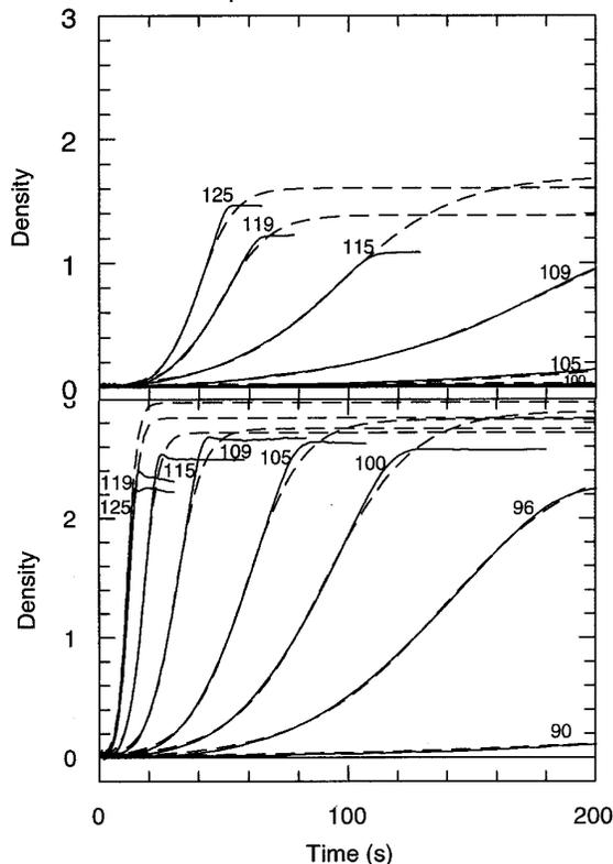
Figure 1. DryView development kinetics (—) and calculated autocatalytic curves (---). Processing of unexposed (top) and exposed (bottom) films was carried out in a fluorochemical bath at the temperature ( $^{\circ}\text{C}$ ) indicated next to each curve. Density was measured at 1000 nm.
