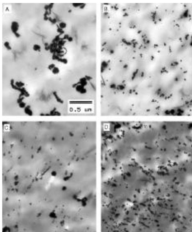
Figure 5. Electron micrographs of silver particles in photothermographic systems containing no infectious developer (A), II (B), I (C), and III (D). These electron micrographs are at a magnification of 30,000 and show a representative portion of the complete electron micrograph.
