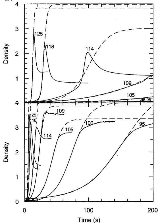
Figure 2. Photothermographic development kinetics (—) and calculated autocatalytic curves (---) for a high contrast film containing Nonox and II at a 1:1 ratio at the development temperature ( $^{\circ}\text{C}$ ) indicated next to each curve. Both unexposed (top) and exposed (bottom) films are shown. Density was measured at 1000 nm.
