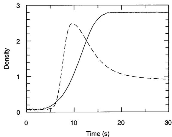
Figure 3. Development kinetics at  $125^{\circ}\text{C}$  in a fluorochemical bath for photothermographic films without infectious developer (—) and containing **IV** at a ratio to soap of 0.0015 (---). Density was monitored at 1000 nm.
