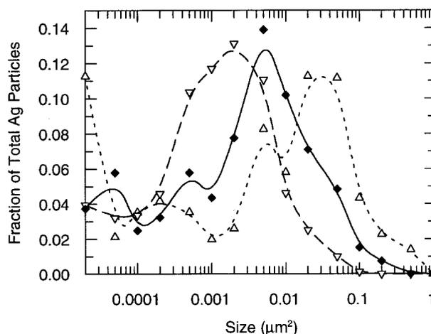
Figure 7. Particle size distribution for various development systems including standard development (Δ), high contrast infectious development (∇), and low contrast infectious development (◆). The particle size distribution for high contrast infectious development represents the average for formulations containing I, II, and III. The sum of the fraction of total silver particles is 1.00 for each curve.
