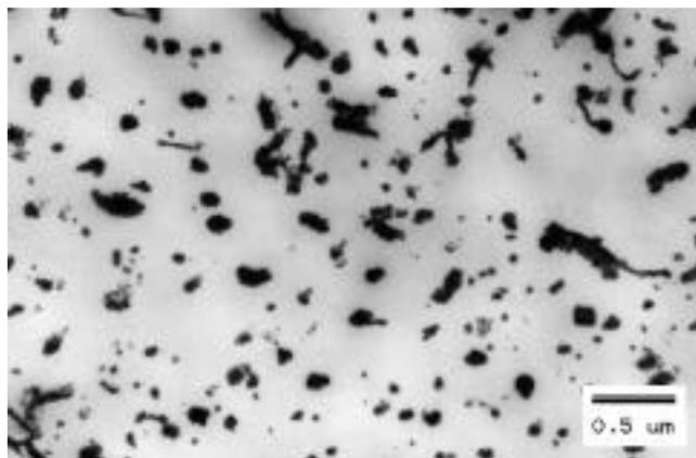
Figure 6. Electron micrograph of photothermographic film containing a low level of IV. The codeveloper to soap ratio was 0.00147, with a coating weight of 1.54 g Ag/m<sup>2</sup>.
