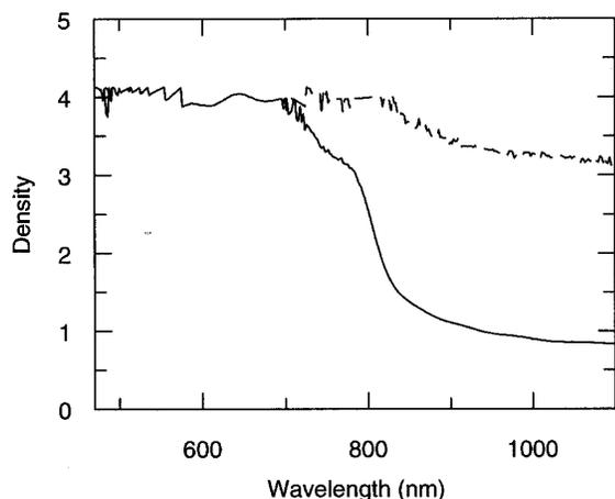
Figure 4. Spectral absorbance of high contrast film (—) and DryView (---). Films were exposed for 5 s at an intensity of 1 on a 3M Model 179 Contact Printer-Processor and developed for 15 s at 124°C. Films developed for 23 s showed similar absorbances.
