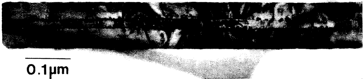
Figure 2. Cross-section image of AgBr/AgBrI platelet showing the existence of internal (111) twin boundaries. Secondary twin bands are occasionally found in the upper(or lower) primary twin regions. They have now been detected in the middle twin region.
