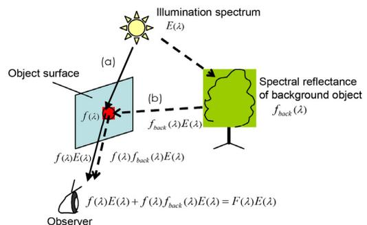
Figure 2. Model of reflection light in the proposed method. .
