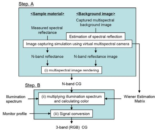
Figure 3. Diagram of multispectral CG rendering.
