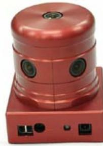
Figure 4. Camera head of omni-directional camera .
