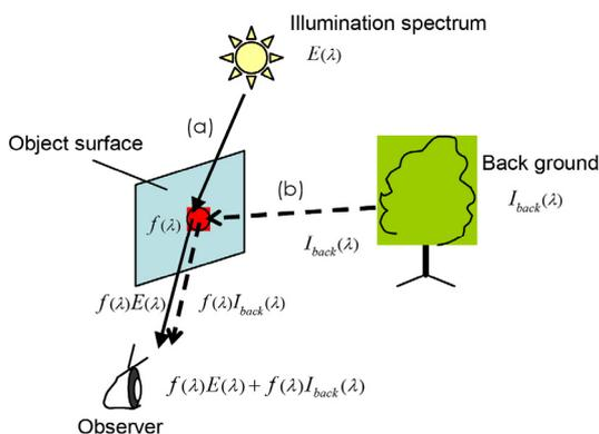
Figure 1. Model of observed reflection light.
