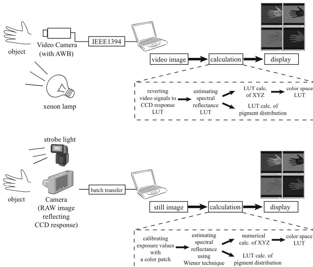
The lower diagram is the prototype and the upper diagram is the modified one.
