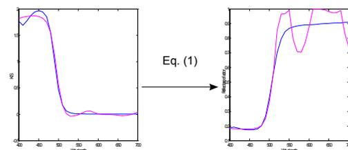
Figure 1. An example of enhanced R space spectral error reconstructed in  $\Phi$  space by the Kubelka-Munk transformation of Eq. (1)
