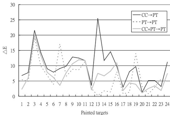
Fig. 2. Testing results for all painted targets by using the pseudo inverse model (No. 13 is the blue color referred in Fig. 1).
