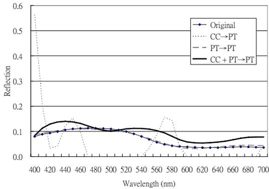
Fig. 1. Reflectance curves of the original, the first estimated (CC→PT), the second estimated (CC→PT), and the third estimated (CC+PT→PT) spectral values for a blue color in painted Oriental water color by the pseudo inverse model.
