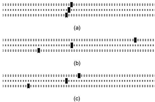
Figure 2. The Hinton diagrams of selection matrices. a)  $\mathbf{W}$  for  $PI_s$ , b)  $\mathbf{W}$  for  $PI_c$  and c)  $\mathbf{W}$  for  $PI$ . The zero-valued elements are shown by small squares. The unit elements are shown by black squares. A horizontal position of elements corresponds to wavelength from 400 to 700 nm taken at 5 nm. The first, second and third row in each diagram define the selected R, G and B components, respectively.
