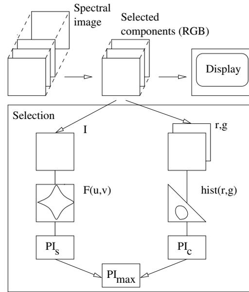
*Figure 1. The generic RGB color fusion scheme and the flow chart of the proposed component selection method.*
