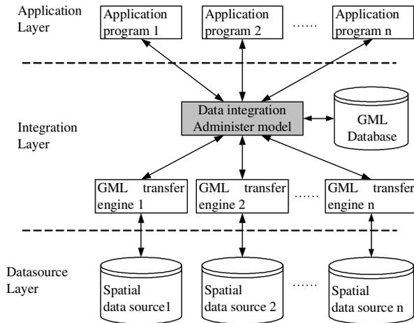
Figure 2 GML based multi-source spatial data integration model
