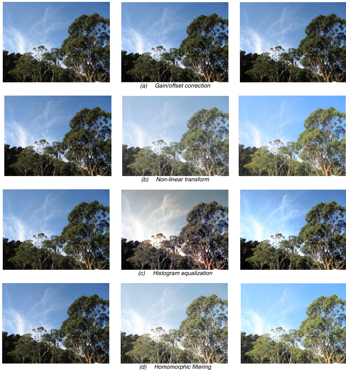
Figure 2. Color image enhancement (left) with (right) and without (middle) color characterization, enhancement, and color balancing
