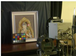
Figure 4. Multispectral image acquisition experiment using a 16-band camera.
