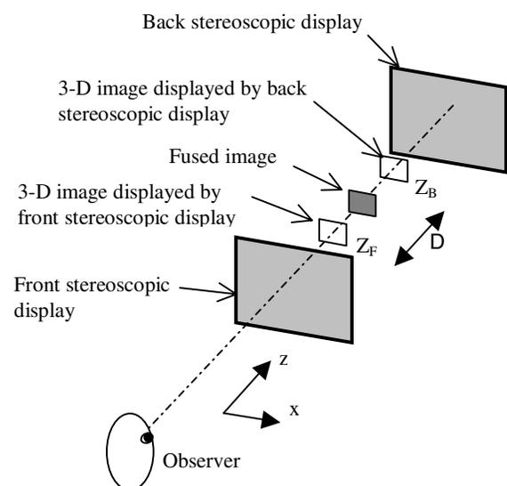
Figure 1. Schematic of new 3-D display system.  $Z_F$  and  $Z_B$  indicate original perceived depth of 3-D images displayed by front and back stereoscopic display, respectively, which means perceived depth of 3-D image when each display shows 3-D image alone.
