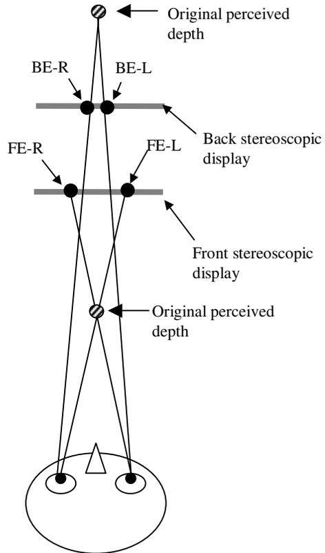
**Figure 5.** Position of pattern edges for left and right eyes on stereoscopic display and perceived depth of 3-D image. FE-R and FE-L indicate pattern edges of images for right and left eyes displayed by front stereoscopic display. BE-R and BE-L indicate pattern edges of images for right and left eyes displayed by back stereoscopic display.
