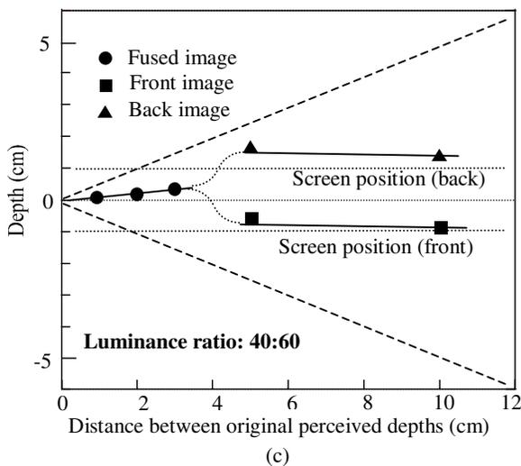
**Figure 4.** Results of subjective tests on perceived depth of 3-D images. Differences between three graphs are in luminance ratios of front and back 3-D images.
