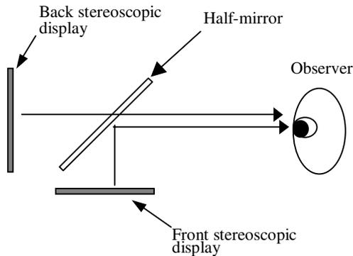
Figure 2. Optical configuration used in experiment.
