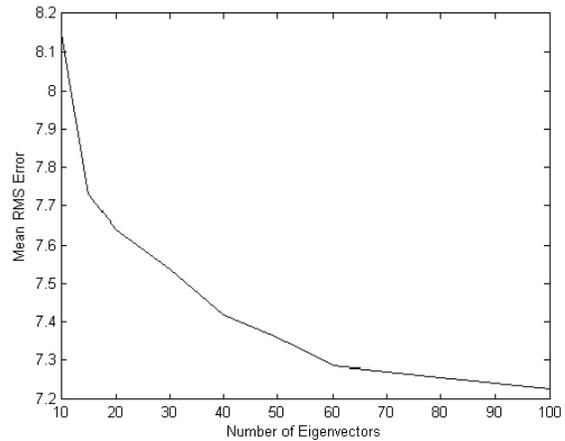
Figure 3. Mean RMS error using different number of eigenflows. Mean RMS error of the original images was 70.51.
