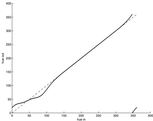
Fig. 2. The resulting effect of the hue squeezing using the double-Gaus method. The double-Gaus method more gradually compresses near the preferred hue angle than a single-Gaus function.
