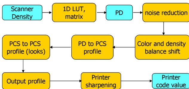
Figure 2. Image processing for scenes originating on film.
