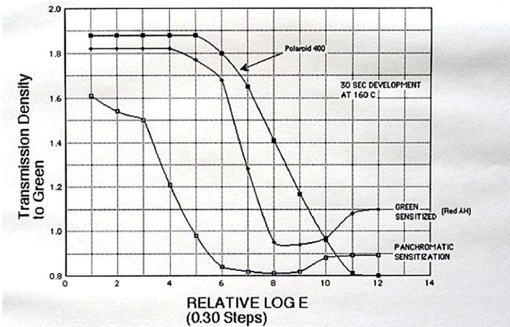
Figure 3. Comparison of sensitometric responses of Polaroid 400 with green sensitized and panchromatically sensitized, photothermographic reversal experiments.
