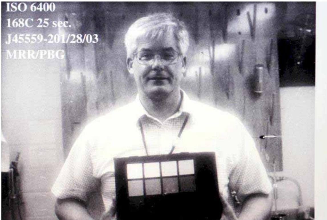
Figure 2. ISO 6400 test exposure with green sensitized photothermographic layer, fluorescent lighting with grayscale chart.
