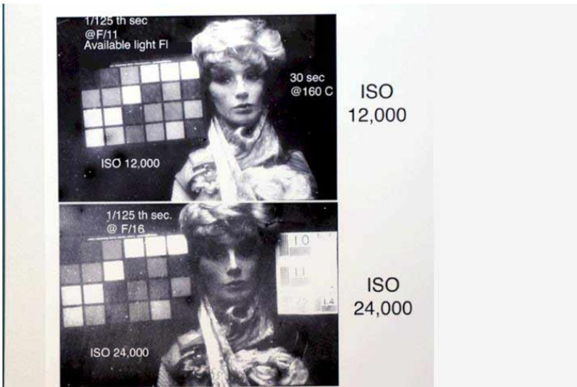
Figure 4. Picture tests of panchromatically sensitized coatings at ISO 12,000 and ISO 24,000.
