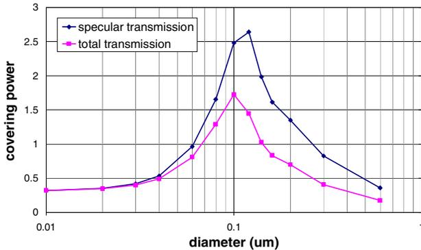
**Figure 2.** Calculated covering power for solid silver spheres dispersed randomly in a 20  $\mu\text{m}$  layer with a silver loading of 1.9  $\text{g}/\text{m}^2$ .
