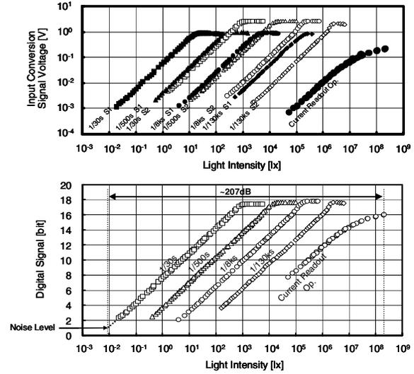
Figure 5. Photoelectric conversion characteristics [25].
