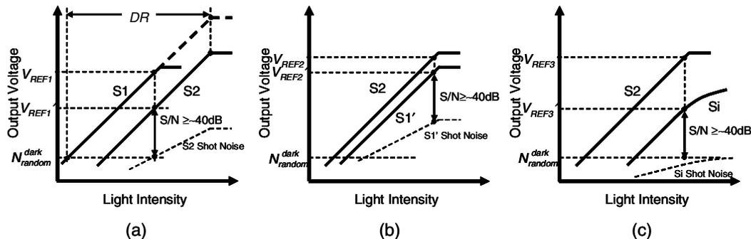
Figure 4. Signal switching methods (a) in one voltage readout operation. (b) in two successive voltage readout operations. (c) between voltage readout operation and current readout operation.
