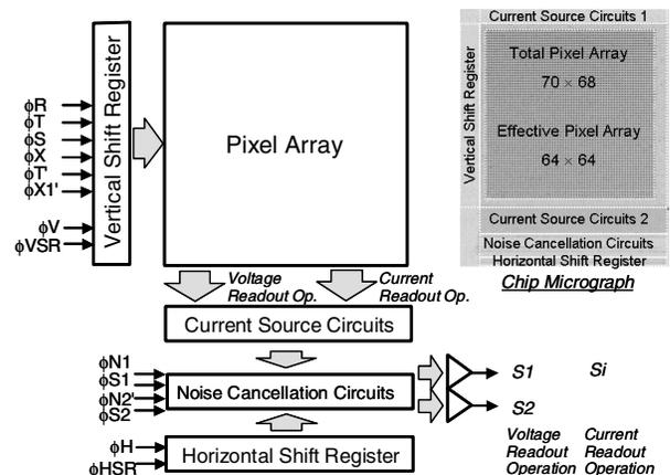
Figure 2. Block diagram and chip micrograph [25]. The chip size is  $2.6 \times 2.6 \text{ mm}^2$ .
