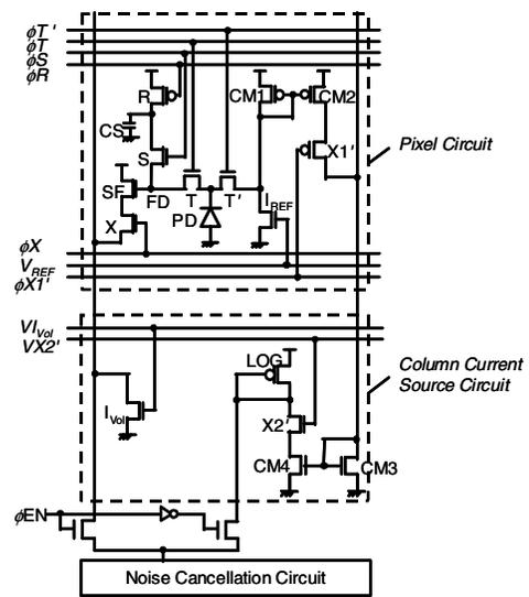
Figure 1. Schematic diagram of a pixel and a column circuit [25].
