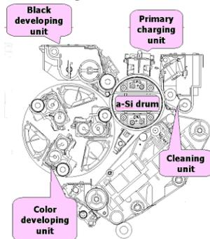
Fig.1 Cross section of imageRUNNER™ C6800 marking engine
