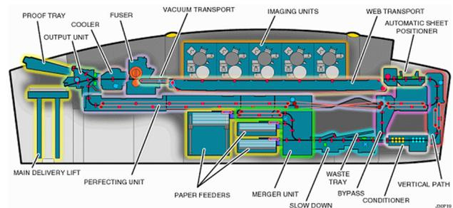
Figure 1. NexPress 2100 digital press equipped with 5 print units.
