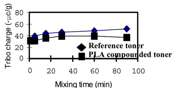
Figure 2. Electrostatic Charge by time
