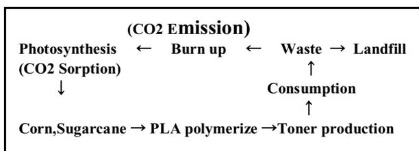
Figure 1. Environmental cycle of PLA used in toner.
