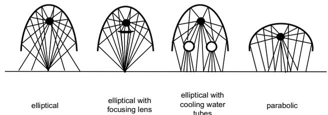
Figure 3. Typical Reflectors
