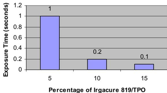
Figure 4. Cure speed versus phosphine oxide photoinitiator content.
