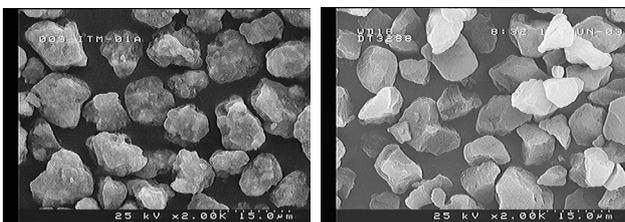
Figure 1. SEM image of and ceramic(left) and conventional toner (right)
