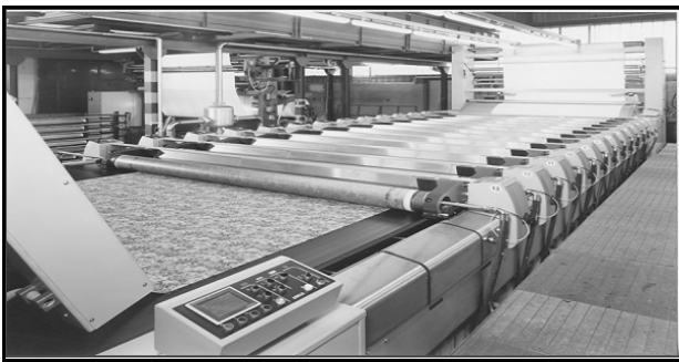
Figure 1. Reggiani Macchine S.p.A. rotary screen printing machine
