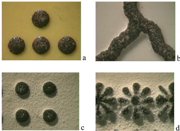
Figure 3. Microscopic view of swell paper features. (a) Braille dots, (b) lines from a tactile diagram, (c) Braille dots deformed in transport and (d) poor swelling due to excessive temperature.
