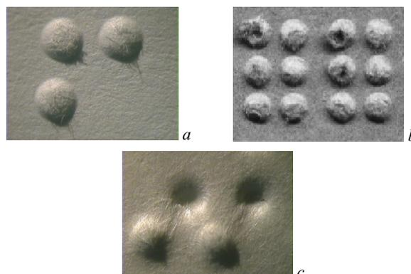
Figure 1. Enlarged view of embossed Braille characters; (a) good printing (single sided), (b) poor printing (defected dots), (c) double sided printing.
