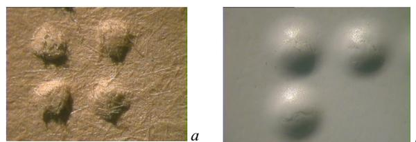
Figure 2. The shape of Braille dots on (a) rough paper and (b) a quality smooth paper.
