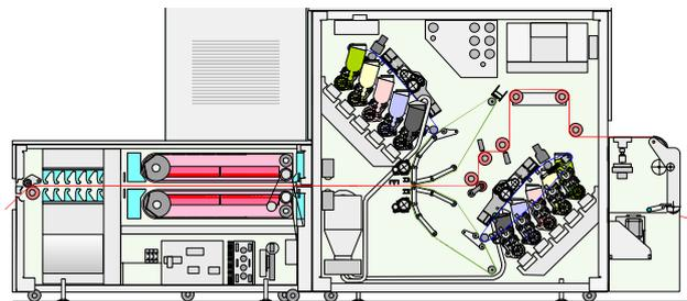
Figure 2. VS 9000 paper input, print module and fusing module
