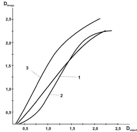
Figure 2. Tone reproduction curves in hybrid photographic systems: 1-silver halide process, 2-system with scanning a negative, 3-shooting by the digital camera.
