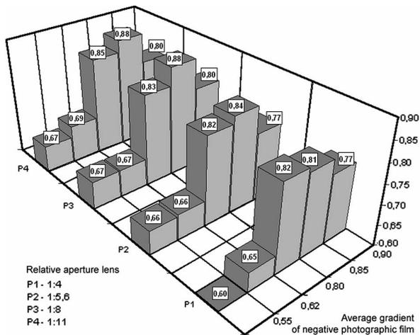
Figure 5. Relation of general gradient of the tone-reproduction curve to the gradient in half-tones versus values of the relative aperture lens and average gradient of negative photographic film
