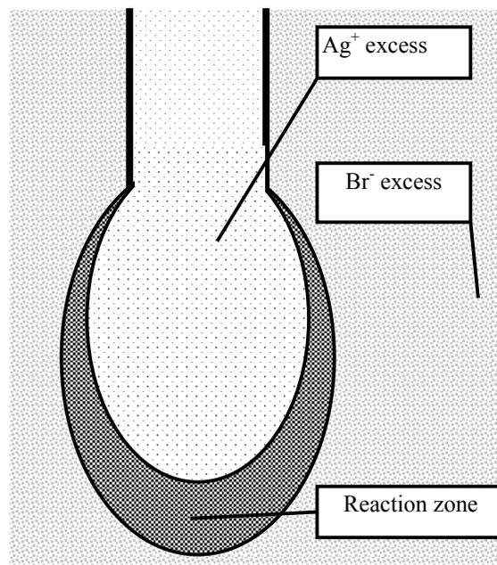
**Fig. 1.** The distribution of different zones when introducing the silver nitrate solution into a reaction mix (the solution containing a bromide ion excess).
