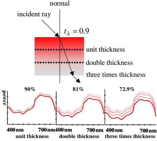
Figure 3. Reduction in energy of transmitted light according to object thickness
