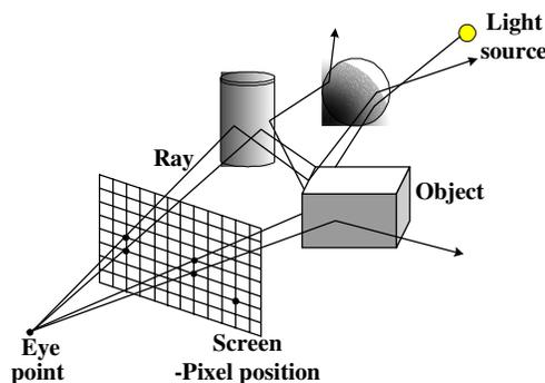
Figure 1. Concept of backward ray tracing
