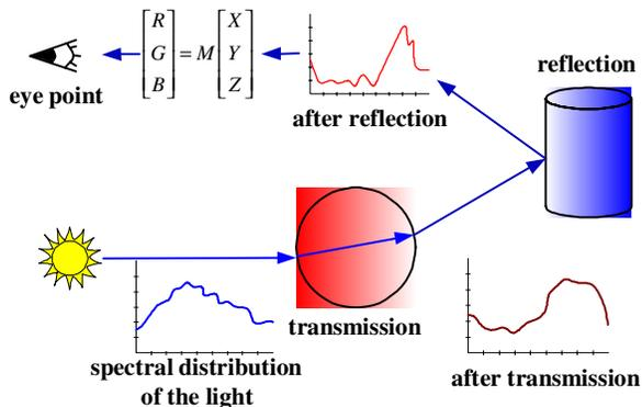
Figure 2. Calculation of color based on spectral distribution of light sources and objects
