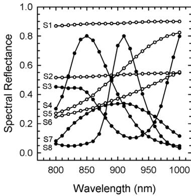
Figure 2. Spectral reflectance curves of 8 representative samples belonging to the matrix **Or**.
