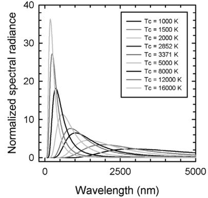
Figure 4. Spectral radiance of the analyzed illuminants normalized to  $10^5$  W/sr\*m<sup>2</sup>.
