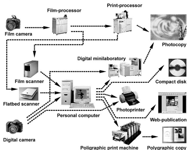
Figure 1. Photographic systems scheme with digital image processing.
