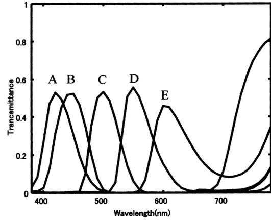
Figure 2. Spectral transmittance of five filters used multi-band camera
