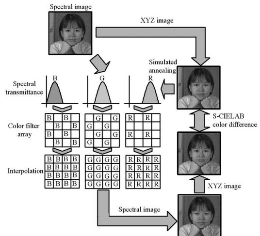
Figure 6. Schematic diagram of filter optimization process
