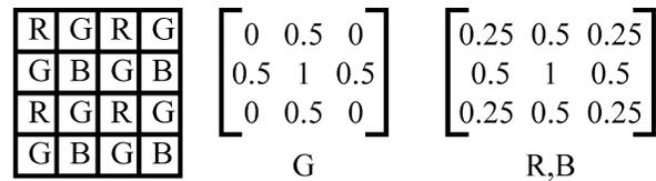
Figure 5. Bayer type color filter array and bi-linear interpolation
