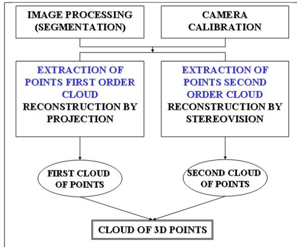
Figure 1: Synoptic scheme of the acquisition system.
