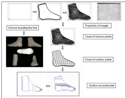
Figure 7: Surface Reconstruction Method.
