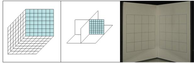
Figure 3: The calibration pattern used.
