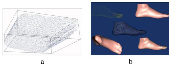
Figure 8: a : first cloud of points, b : surface modelling.
