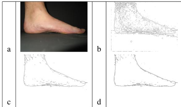
Figure 4: Contour extraction, a : original image, b : Laplacian, c : Sobel, d : Roberts.
