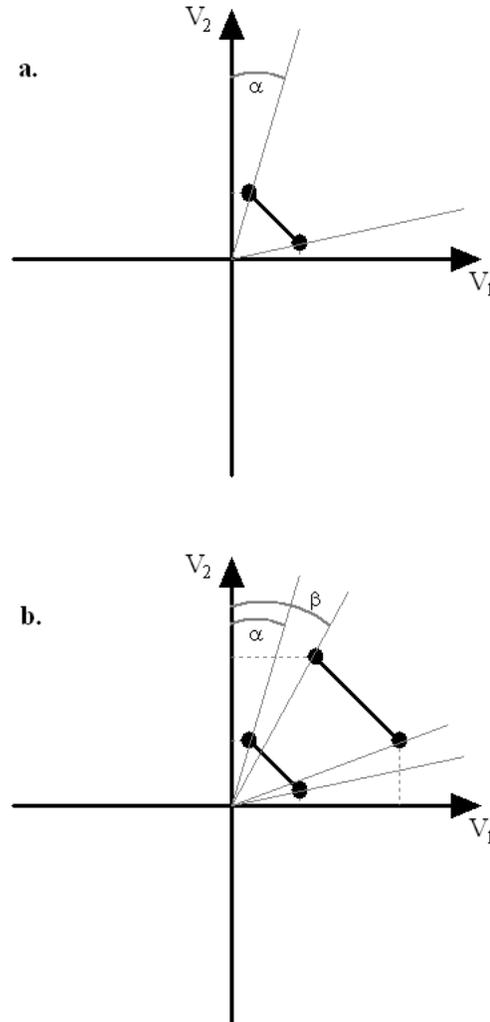
Figure 4. (a) Two colours which are nearest to different eigenvectors in the sense of angular distance may still be close to each other. (b) Colours which have maximum absolute coordinate on those eigenvectors may be more spaced.
