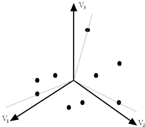
Figure 3. A fictional example of three eigenvectors and nine target colours. The colours nearest to each eigenvector in the sense of angular distance are marked.
