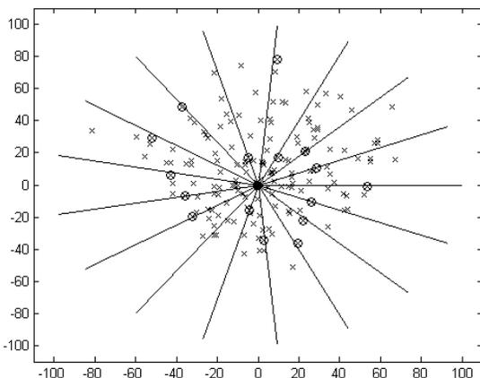
Figure 1. An example of how training set colours are chosen in the HC plane. The central half-lines of all the sectors are drawn, and the chosen colours are circled.
