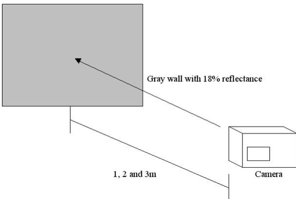
Figure 2. Experiment setup for energy table
