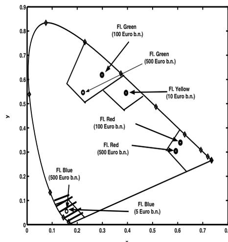
Figure 3. The CIE 1931  $x,y$  diagram, luminescent colors used in Euro banknotes plotted. Approximate areas of used luminescent colors are marked around the measured example colors.
