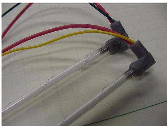
Figure 8. Lamps Wrapped with Instant Lamp Warmup Wiring
