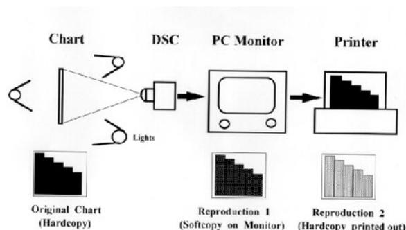
Figure 4. The procedure of the tonal characteristic analysis
