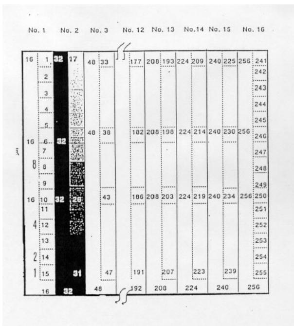
Figure 1. The pattern of the 8 bits linear lightness chart
