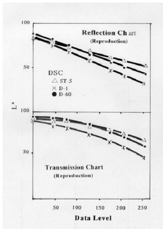
Figure 5. The  $L^*$  value change on the reproduced chart images on the PC monitor.
